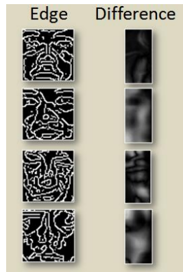
Figure 3 Intermediate images of face images: significant face edges; difference between left and right face. Source [1].
