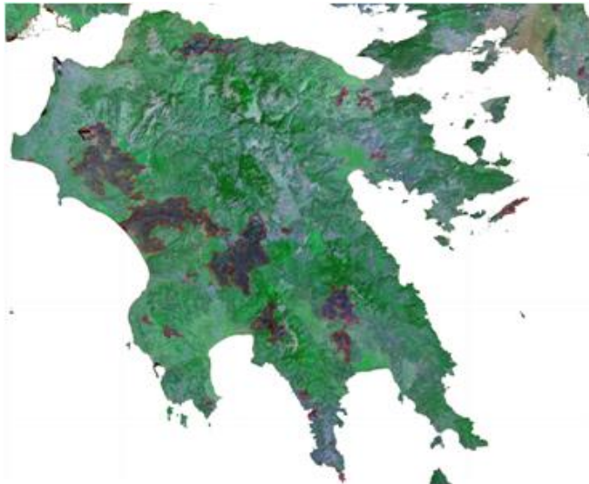
Fig.4 Burnt scars caused by fires in Greece in 2007 mapped from MODIS satellite imagery [10]
